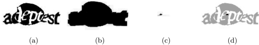
Fig. 3: Ellipse center estimation. After 7 iterations of erosion only one connected component is left 3b. After 58 iterations of dilation only a few pixels close to the center are left over 3c. Figure 3d shows these pixels in relation to the original image.
