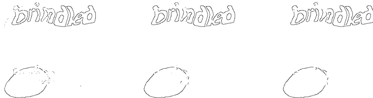
Fig. 4: Cascaded ellipse pixel classification. First row: pixels classified as “not ellipse,” second row: pixels classified as “ellipse.” From left to right: Classification after iteration 1, 4, and 9.
