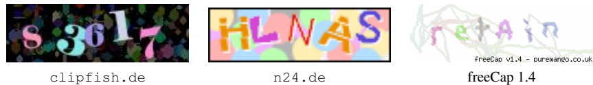
Figure 4: Careless of use of color that makes segmentation and extraction of the characters trivial.
